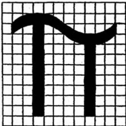
2. The minimum height of the Pi marking shall be 5 mm. For transportable pressure equipment with a diameter less than or equal to 140 mm the minimum height shall be 2,5 mm.
